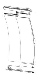
The unit consists of the lower module frame, the lower runner, the glass door, the upper runner, the upper module frame and the assembly kit.
