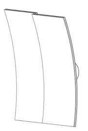
Depending on the version, the sliding glass door is made of 6mm tempered safety glass or 4mm tempered safety glass on the outside and 4mm tempered safety glass on the inside, spaced 8 mm apart.
